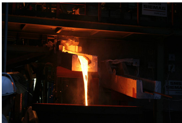
Figure 14. Overflow of the intensive slag-stirring reactor
