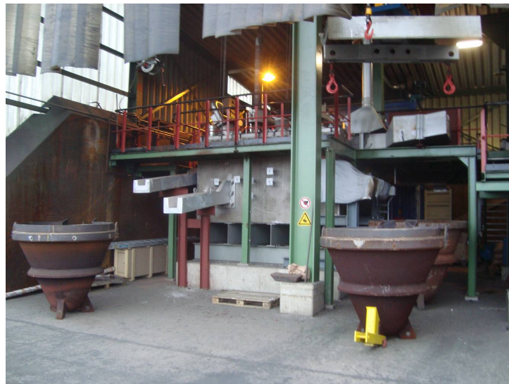
Figure 13. Pilot-scale intensive slag-stirring reactor – front view
