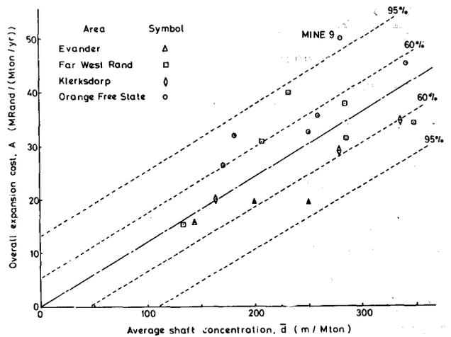
Fig. 8—Coefficient of overall expansion cost plotted against average shaft concentration
