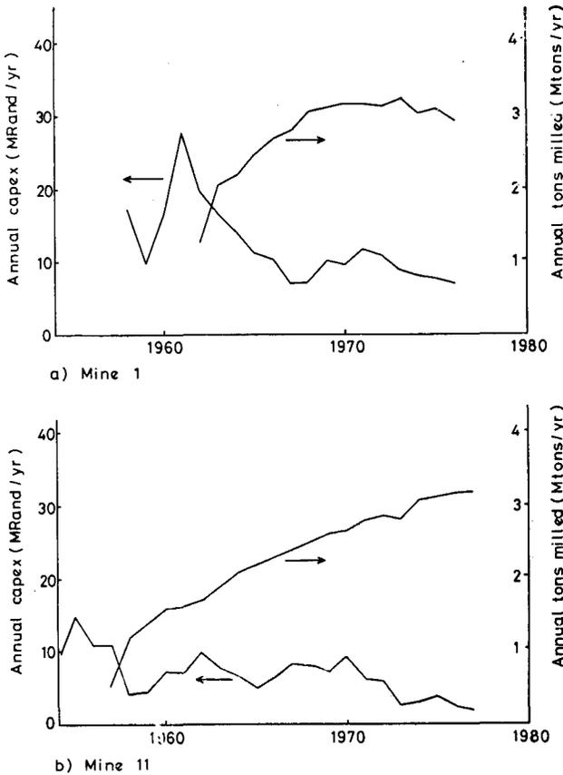
Fig. 1—Annual capital expenditure (1970 basis) and tons milled as functions of time for two mines
