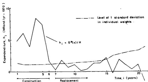
Fig. 5—Average construction/replacement profile estimated for twenty gold mines
