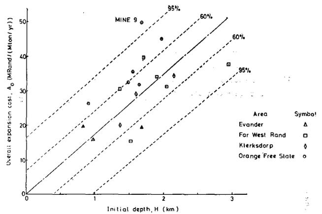
Fig. 7—Coefficient of overall expansion cost plotted against initial depth
