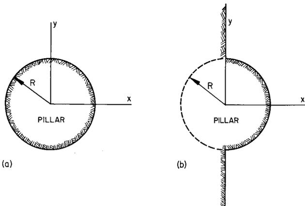
Fig. 2—Most adverse geometries with respect to (a) vertical strain and stress, and (b) tilt
