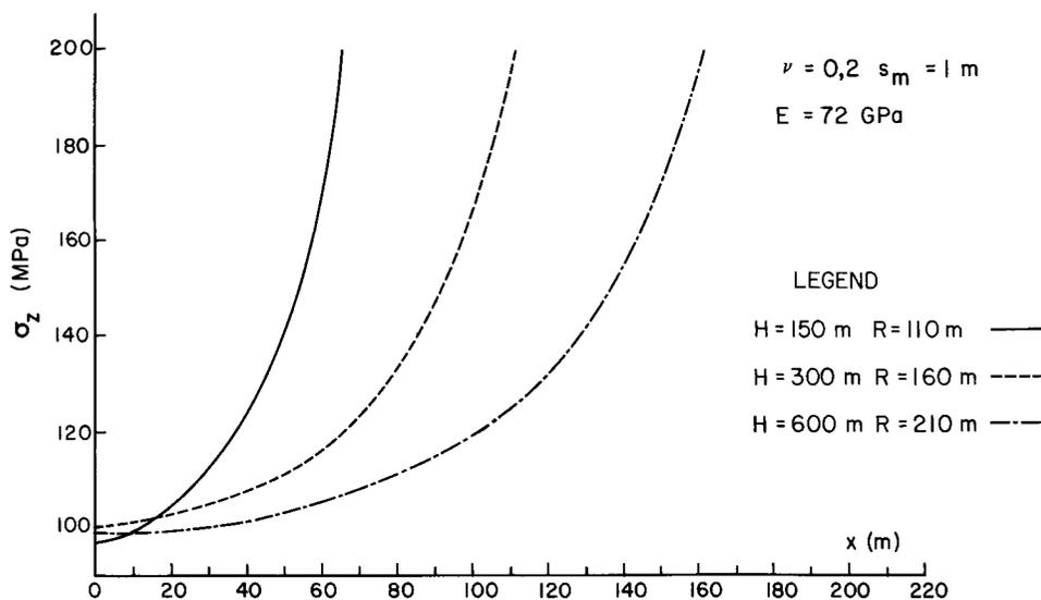
**Fig. 7—Distribution of resultant vertical stress in shaft pillar along a radial line**
