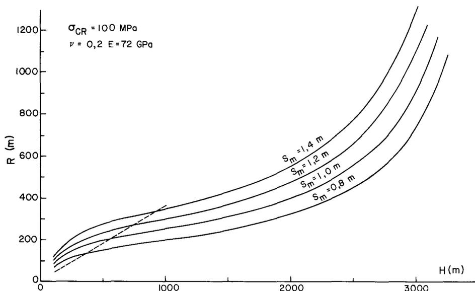
Fig.9—Pillar dimensions for both shallow and deep-level mines and for different stopping widths
