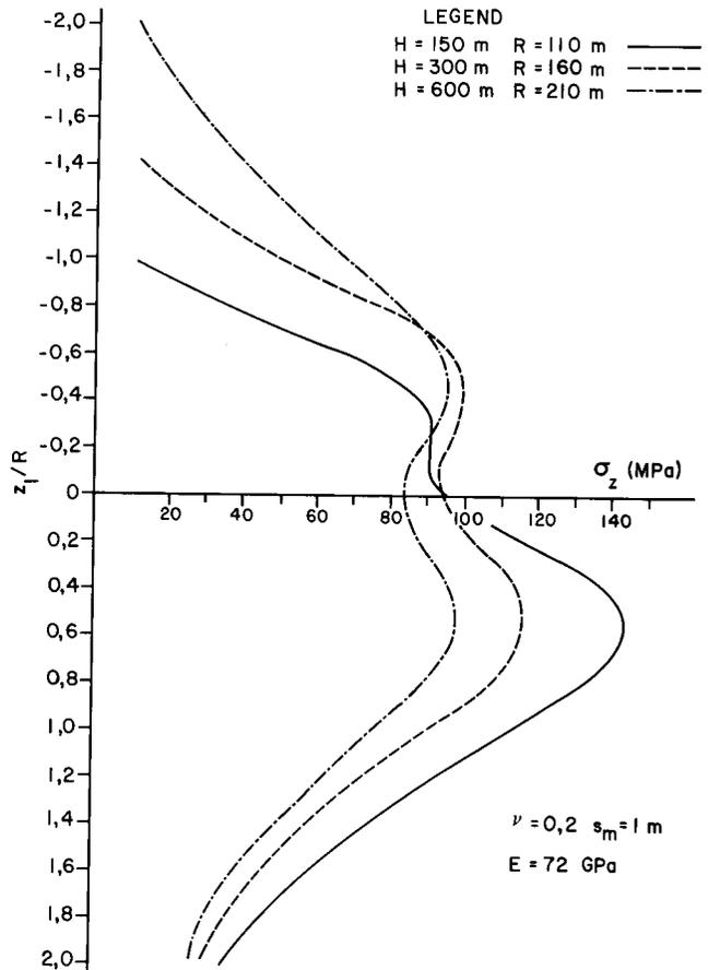
Fig. 6—Distribution of induced vertical stress along the shaft
