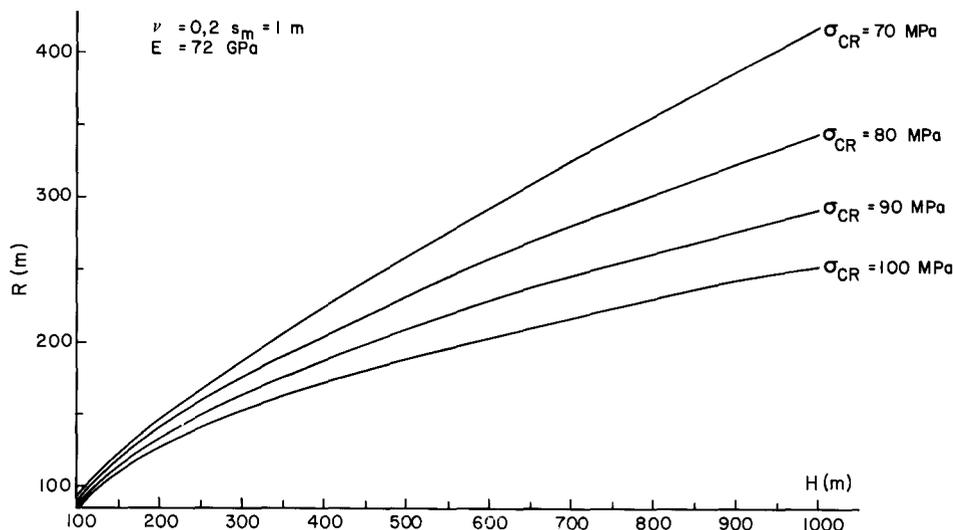
Fig. 8—Pillar dimensions for different critical stresses
