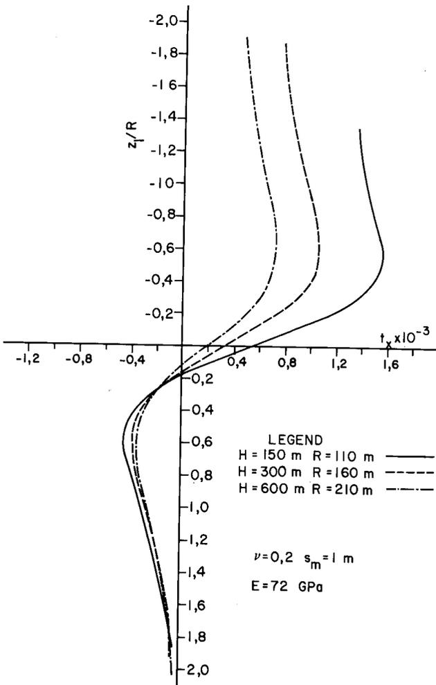
Fig. 5—Distribution of tilt along the shaft
