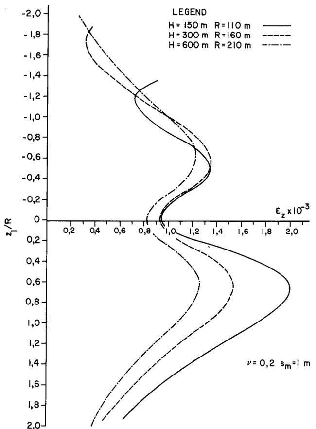
Fig. 3—Distribution of vertical strain along the shaft
