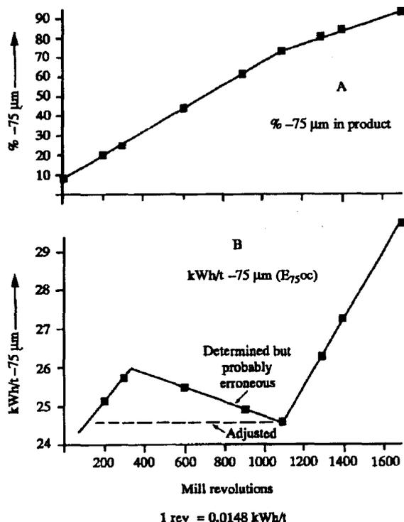
Figure 4—Batch open-circuit test results relating to  $\text{kWh/t} -75 \mu\text{m}$
