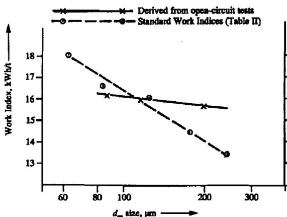
**Figure 5—Standard Work Indices compared with closed-circuit indices derived from open-circuit Work Indices**
