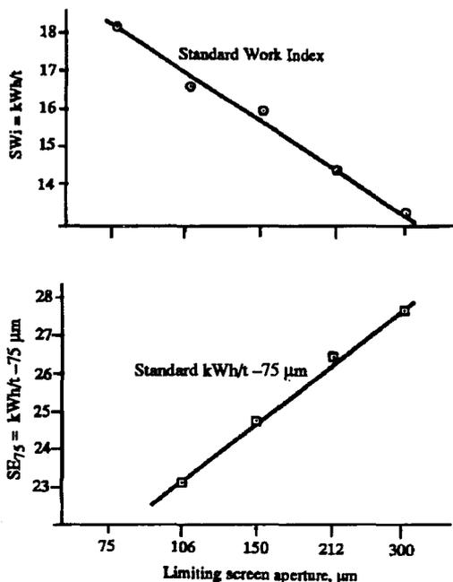
Figure 1—Variation of standard grindability indices with the aperture of the limiting screen
