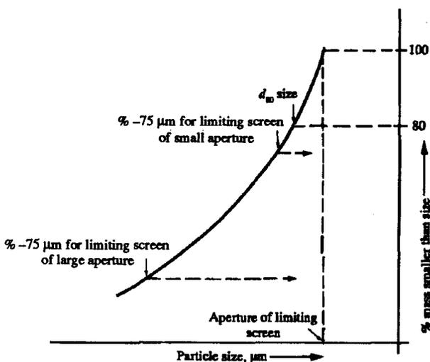
Figure 2—Varying relationship between  $d_{80}$  size and % -75  $\mu\text{m}$  in standard grindability tests
