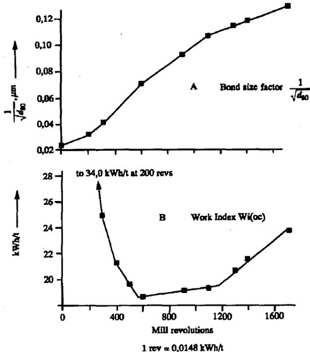
Figure 3—Batch open-circuit test results relating to the Work Index
