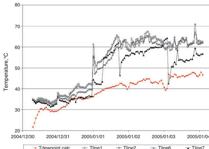
Figure 3—Actual off-gas duct water temperatures. By allowing the cooling-water temperatures to increase, these temperatures were controlled to remain above that of the calculated condensation temperatures
