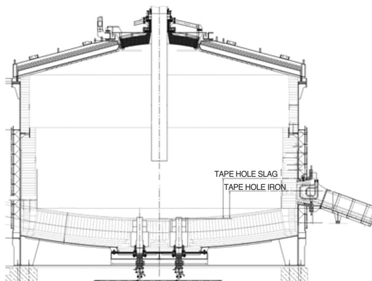
Figure 2—Cross section of the Ticor SA DC ilmenite-smelting furnace
