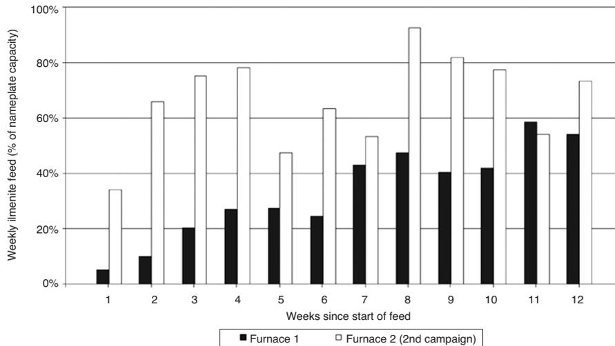
Figure 5—Ramp-up curves—expressed as percentage of nameplate capacity of Furnace 1 and Furnace 2 (second campaign) compared
