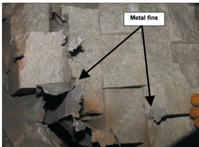
Figure 4—Iron penetration into the hearth found after the refractory break-out of Furnace 2
