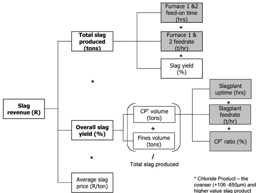
Figure 6—Key performance indicator tree for TiO<sub>2</sub> slag revenue
