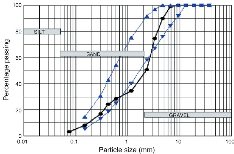
Figure 4—Alpha dust particle size distribution
