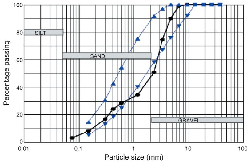
Figure 3—Alpha washed sand particle size distribution
