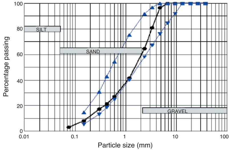
Figure 2—Alpha blended sand particle size distribution
