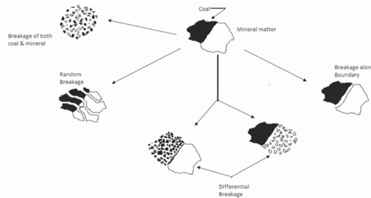
Figure 1—Breakage patterns of coal particles
