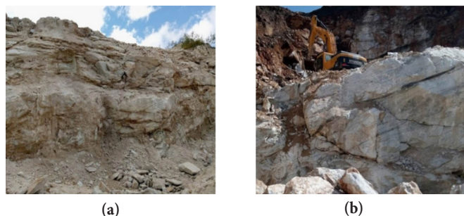
Figure 3—The bench face of (a) Simba and (b) Bisil quarries before blasting showing joint orientation
