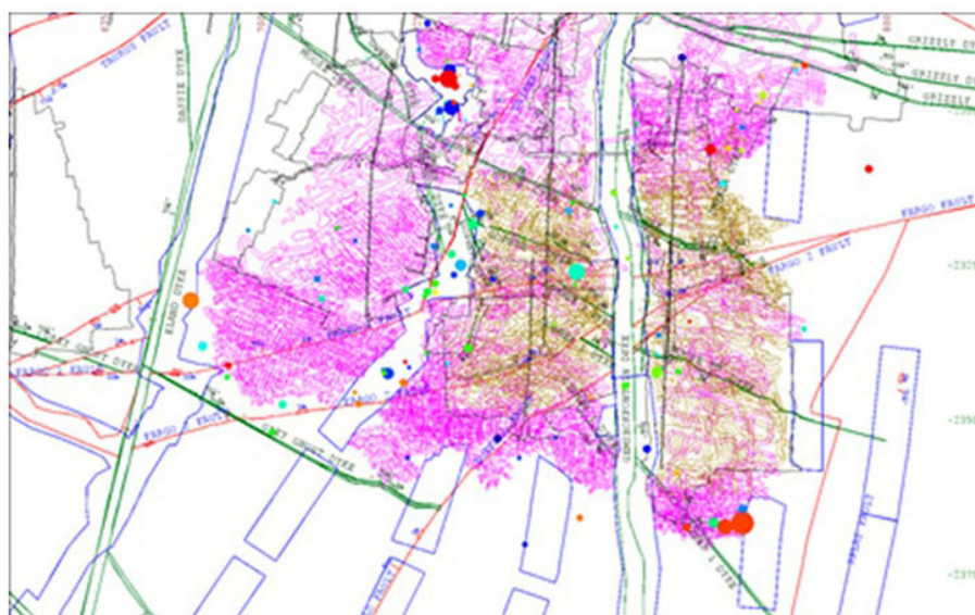
Figure 10—Seismic events after the implementation of destress blasting (Sengani, Zvarivadza, 2017)
