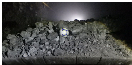
Figure 1—An image of a loaded LHD scoop with a spherical ball added to the payload for the purpose of fragmentation analysis
