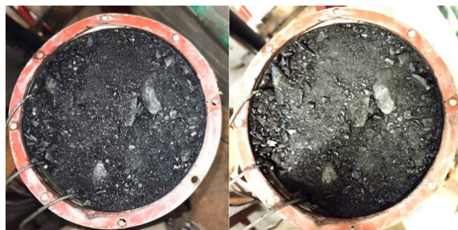
Figure 6—Surface condition of the coal discard specimen (a) before testing and (b) after seepage testing at a hydraulic gradient of e = 0.8 and void ratio i = 1.053
