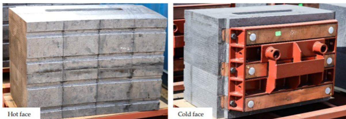
Figure 8—Clad composite copper-graphite cooler with all copper surfaces protected (after Joubert et al., 2024)
