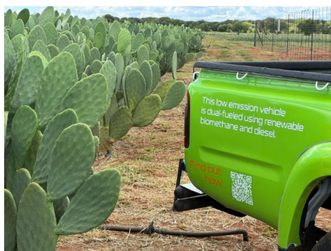
Figure 3. Low-emission vehicle which is dual-fuelled using renewable biomethane and diesel (C-NES, 2024).
