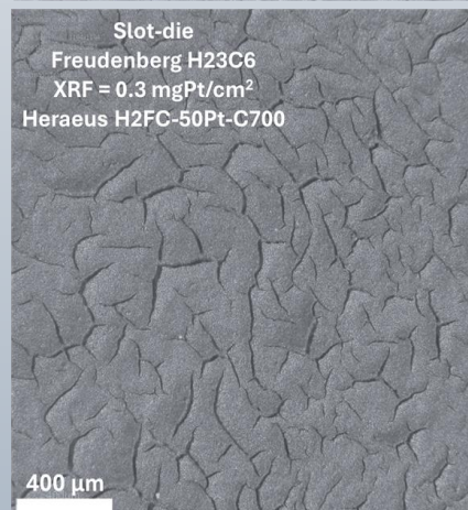
Slot-die coatings on the Freudenberg H23C6 GDL with different Pt/C catalysts
