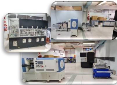
Lab renovated to house intermediate volume MEA production equipment: Roll-2-Roll coater installed in temporary facility
