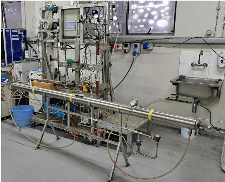
Tests of stage 1 MH container for hydrogen compression
