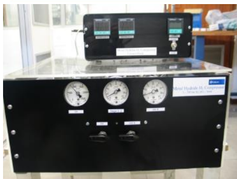
7-200 bar 0.06 Nm 3 /h MH H 2 compressor
