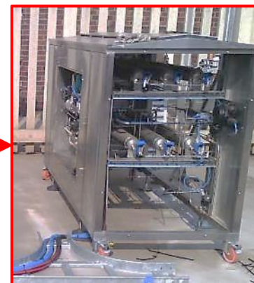
50-200 bar 13 Nm 3 H 2 /h MH H 2 compressor integrated in hydrogen refuelling station
