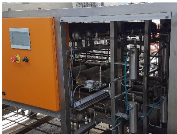
3-200 bar 5 Nm 3 H 2 /h MH H 2 compressor for industrial applications
