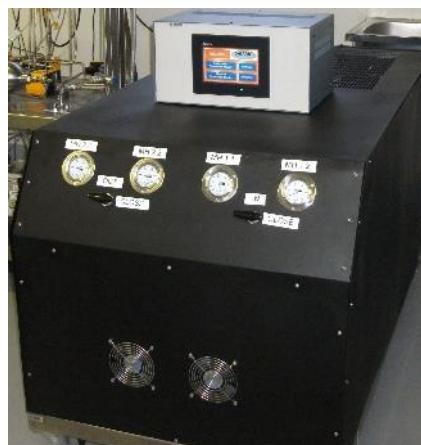
10-200 bar 1 Nm 3 /h MH H 2 compressor
