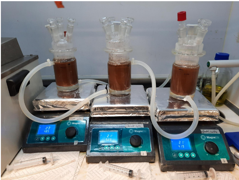
Figure 2. Experimental setup for the leaching process
