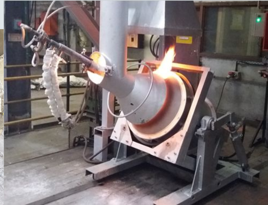
Dynamic refractory testing – TBRC (Chemical and physical wear)
