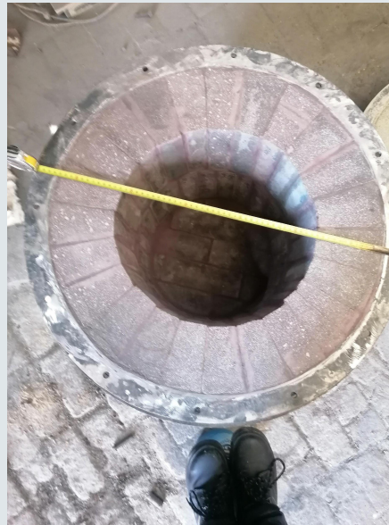
Dynamic refractory testing – TBRC (Chemical and physical wear)
