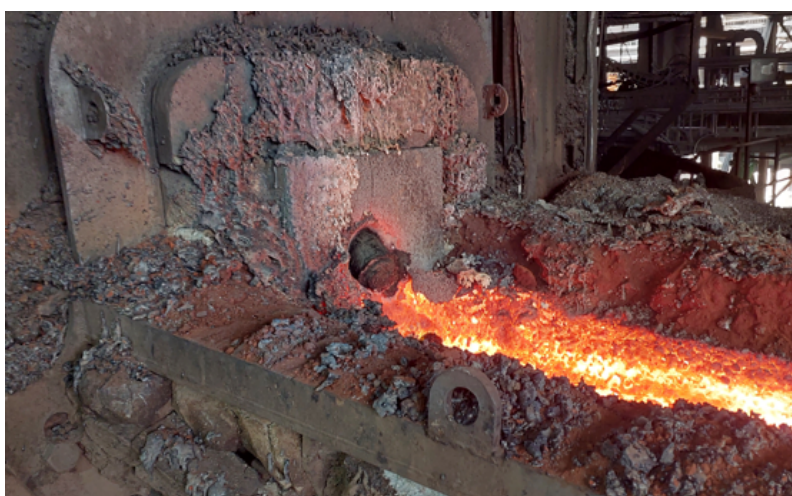
Figure 1: Furnace taphole closed with the synthetic-bonded taphole clay.
