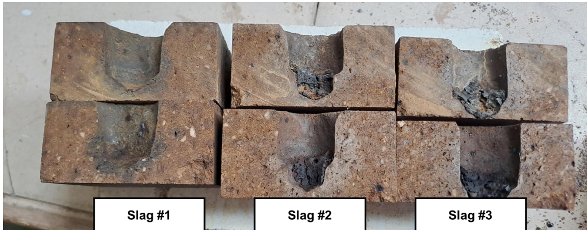
Figure 5. Cup test results for MgO bricks with different slags.
