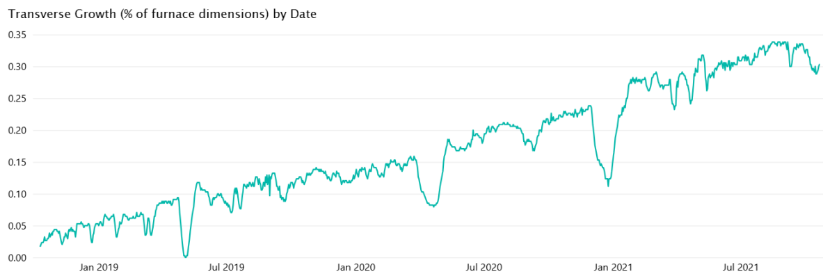
Figure 2. Cumulative transverse (furnace width growth relative to furnace perimeter illustrating typical transverse hearth growth on a PGM rectangular furnace.
