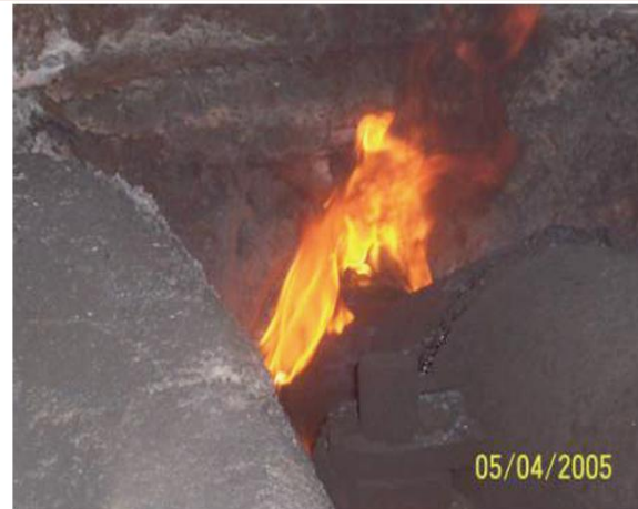
Figure 18. Controlled dosage of tap-hole clay [BM7].
