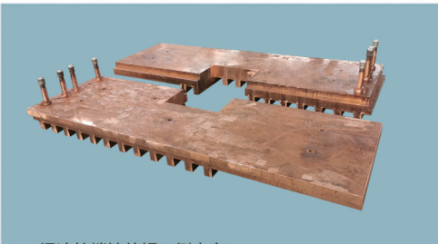
闪速炉端墙放铜口侧水套 end wall copper outlet side water jacket of flash furnace
