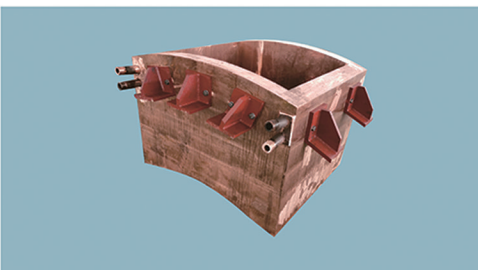
底吹炉烟道口铜水套 smoke passage copper water jacket of bottom blow furnace
