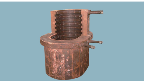
侧吹炉桶溜槽 bucket launder of side blow furnace
