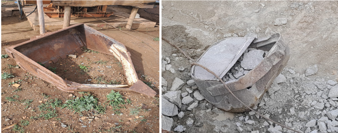
Figure 3: (a) normal scraper scoop (b) modified scraper scoop into a bucket
