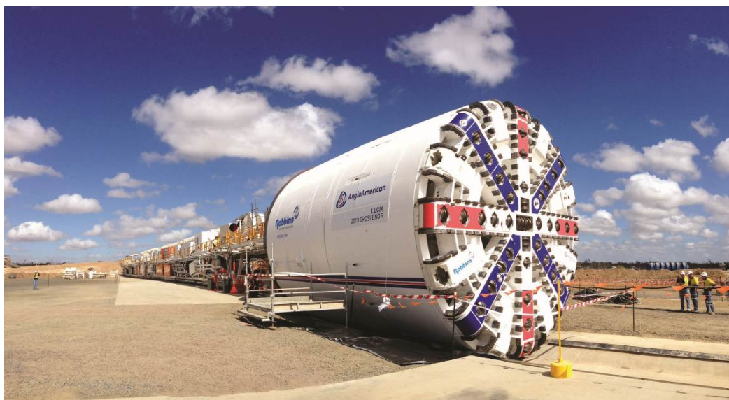
Figure 10: A Robbins Dual Mode EPB/Rock TBM Grosvenor Decline Tunnel Project in Queensland, Australia.
