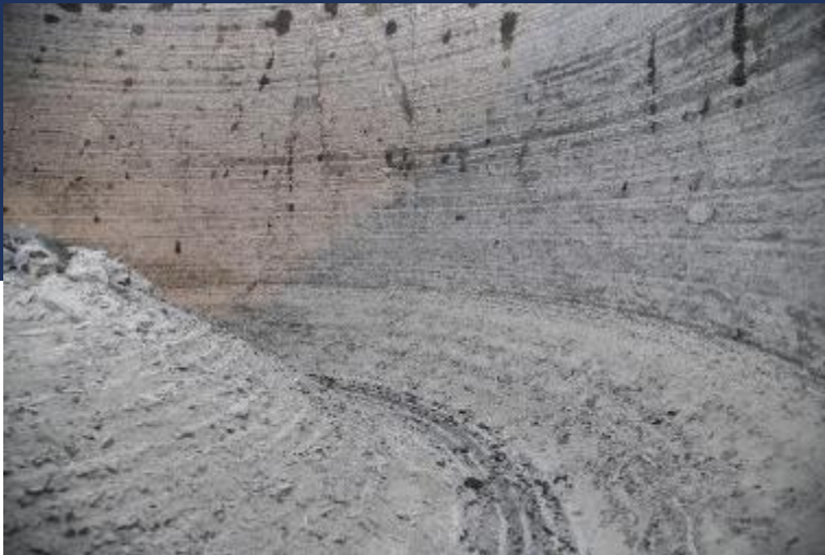
Image: 2019, Concept validation testing 320 MPa rock.
