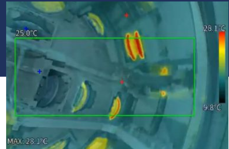
Image: Realtime thermal disk cutter condition monitoring.
