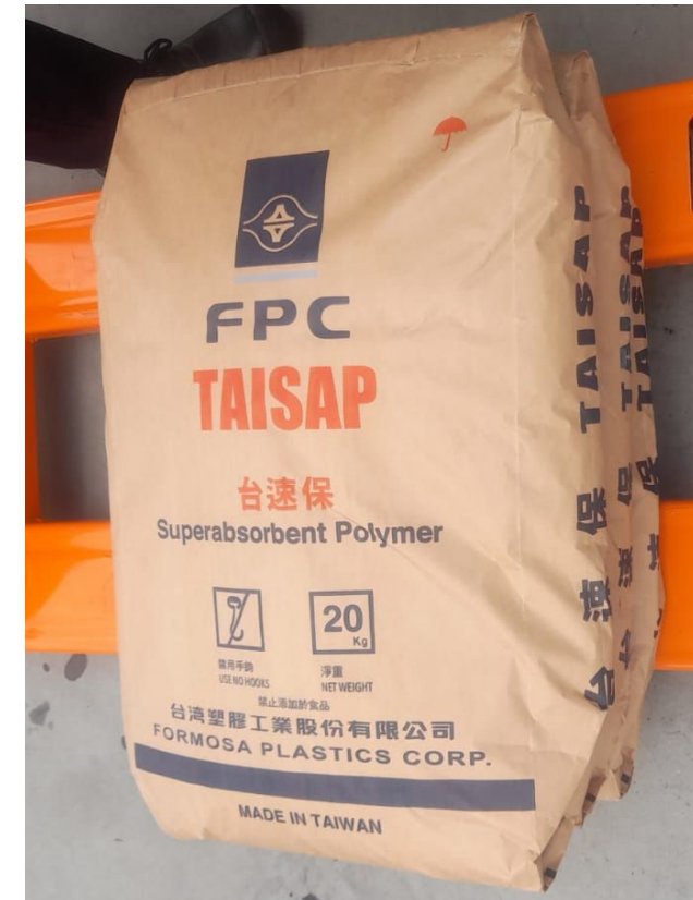
Image 27: Superabsorbent Polymer used to assist in slurry removal
