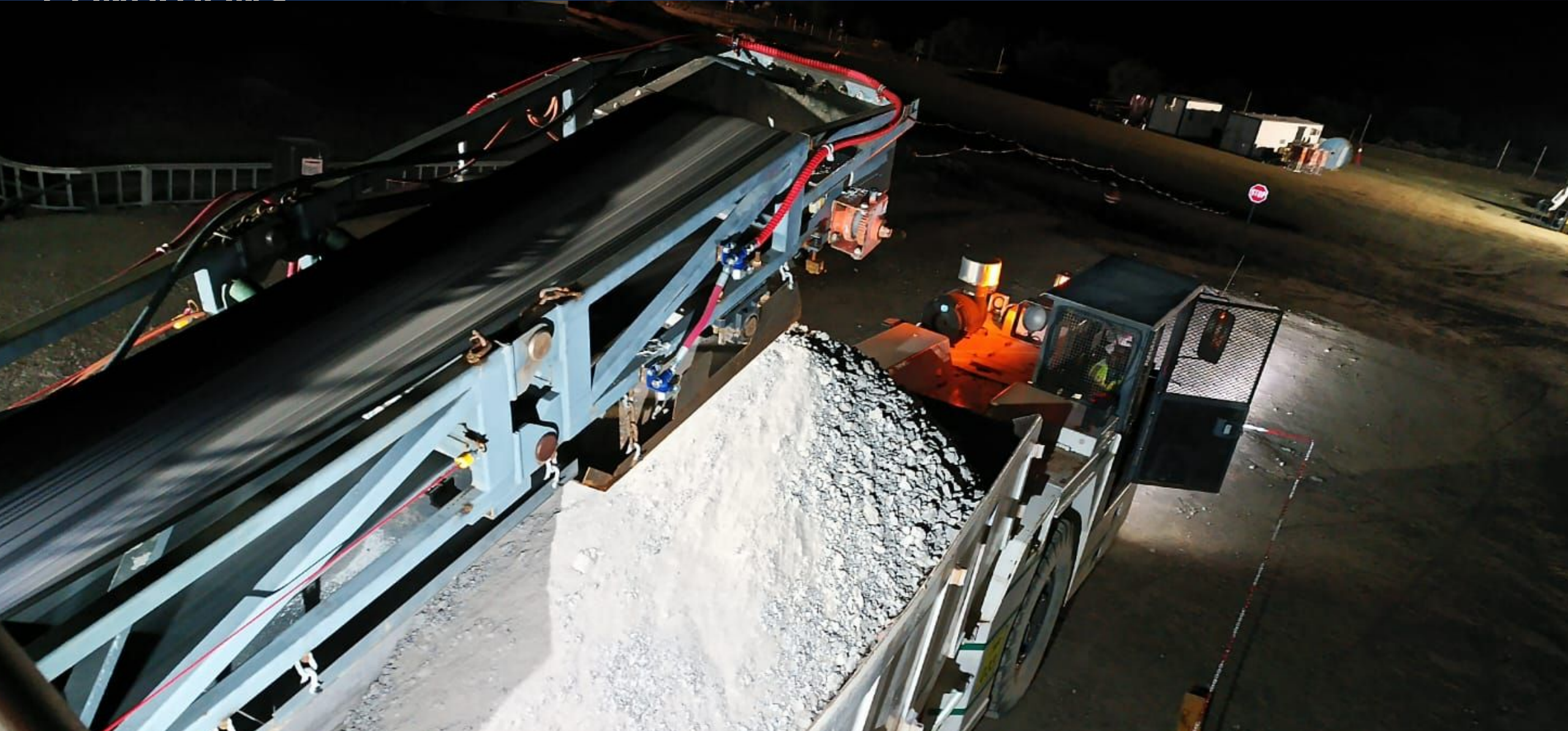
Image 19: MTB collaring, muck in 20-ton dump truck.
