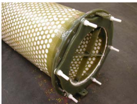
Candle Filter in a GRP + Derakane Resin Structure
