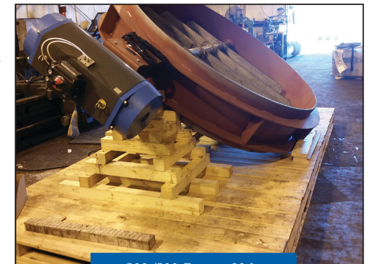
S02/S03 Damper Valves
