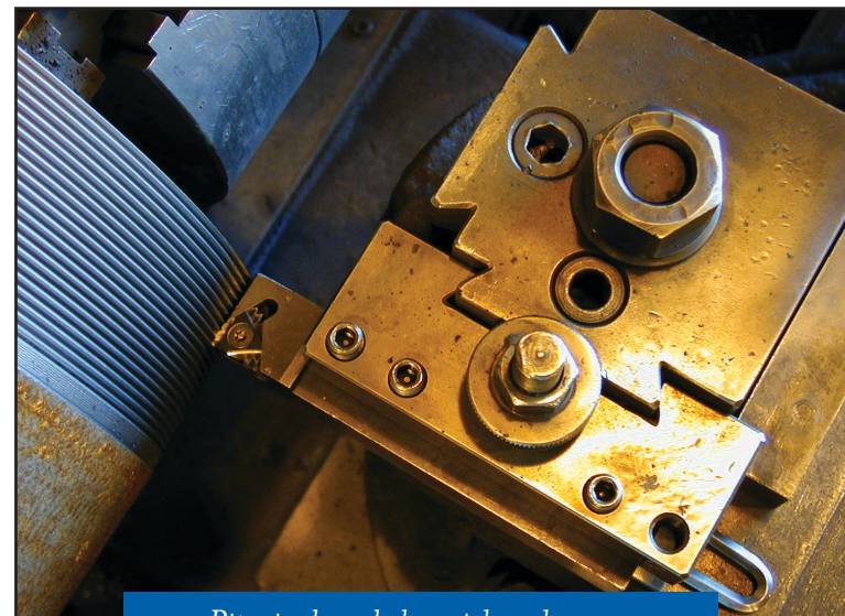
Pipe is threaded to tight tolerances
