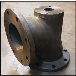
Boss on 90° elbow and Tee for sample or instrument connections at location “Y” and “G”
