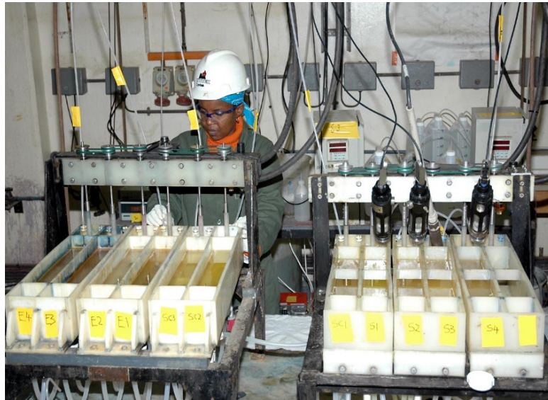
Figure 5: Mintek SX mini-plant.
