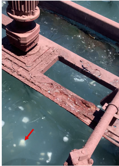
Figure 1. Poor wetting results in the formation of polymer fish-eyes (red arrow) which prevent further water penetration, compromising hydration.
