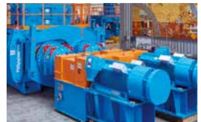
Drive train with motors and gearboxes
