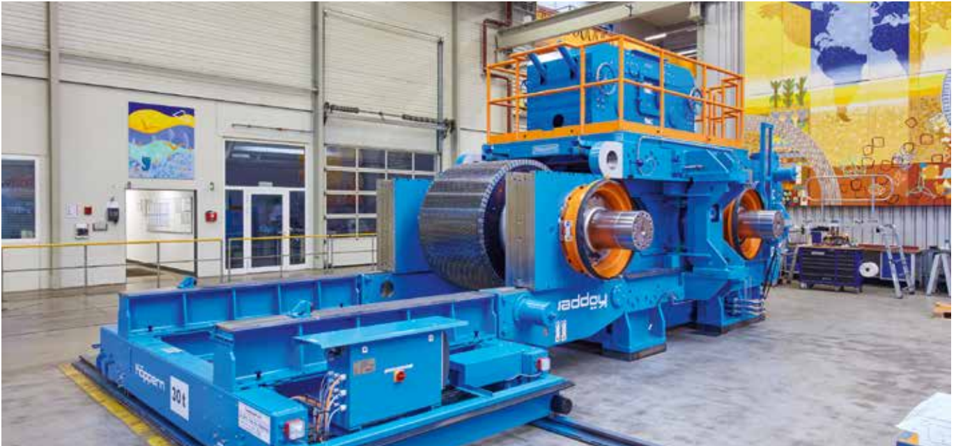
Quick roller change with MHF frame and roller transport carriage
