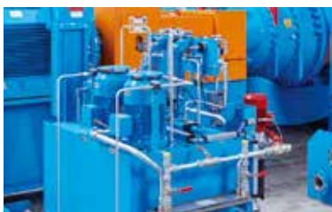
Hydraulic power pack
