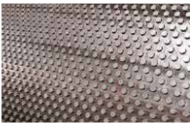
Tire surface with studed wear protection
