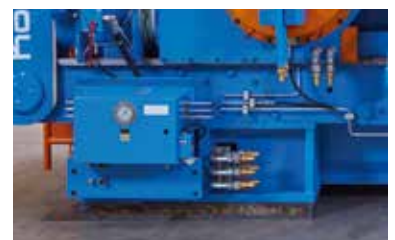
Automatic lubrication system
