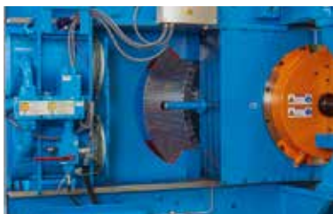
Floating roller and pressurizing cylinders
