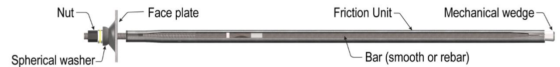
Yielding Mechanical Hybrid Rockbolt
