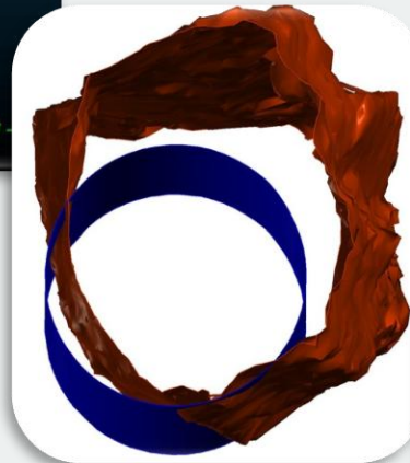
Initial blocky unravelling in dolerite on conclusion of reaming
