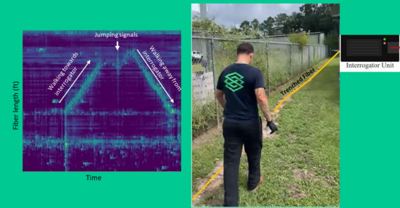
Figure 7. Validation of DAS response to human activity along trenching fibre. Signal patterns correspond to walking toward and away from the interrogator, with distinct acoustic features from jumping events.
