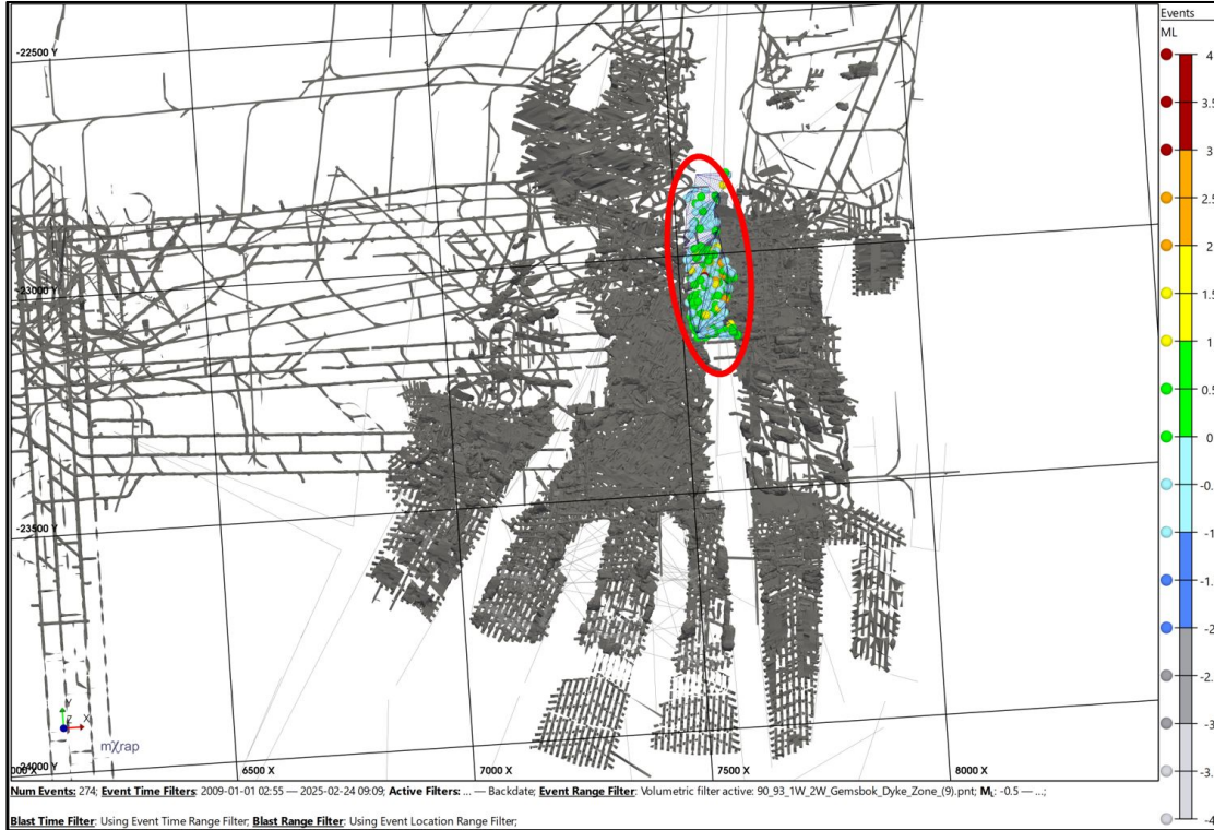
Figure 2: Stability pillar under consideration (area of interest, circled in red) and associated seismic events over 15 years (2009 to 2025).
